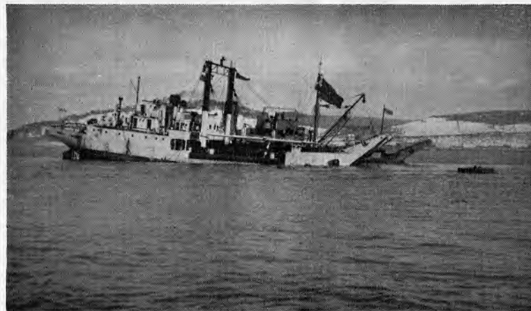
Typical scene of salvage operations. Two salvage vessels 'Pinned' down during a heavy lift on S.S. Gronland in Dover Harbour in 1948.
