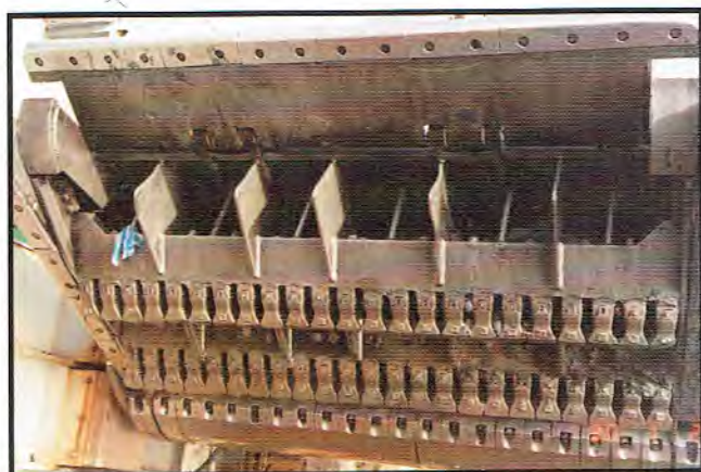
● The Draghead of the Dredger "GEOPOTES 15"
