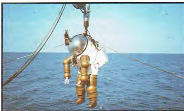
● JIM 22 being swung out prior to deployment. The diver remains at Atmospheric Pressure (1 Bar) throughout the dive.
