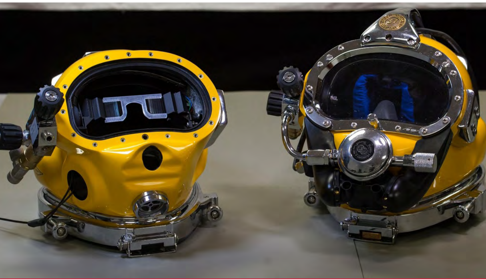
Figure 6: Diver augmented display for enhanced situational awareness.
