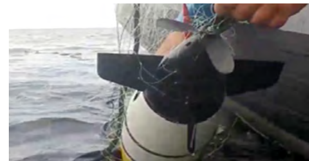
Figure 2: Susceptibility of an AUV to nets as a simple countermeasure.
