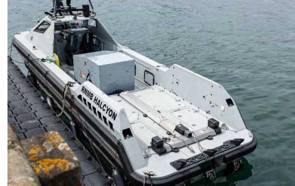
RNMB HALCYON fitted with the sweep system PGM and the removable 'T bar' containing sweep connections and cabling
