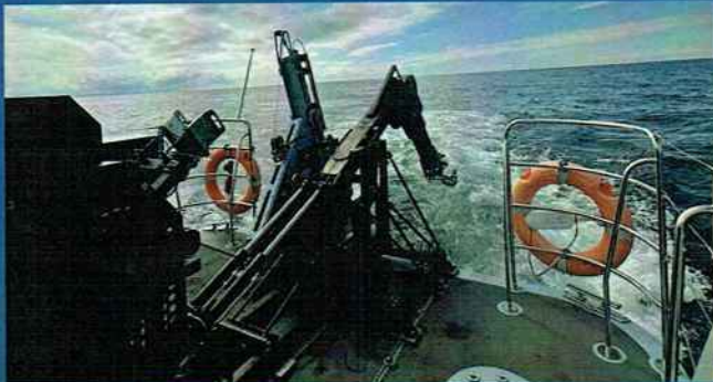
Towed Side Scan Sonar (TSSS) operations from RNMB HEBE.
