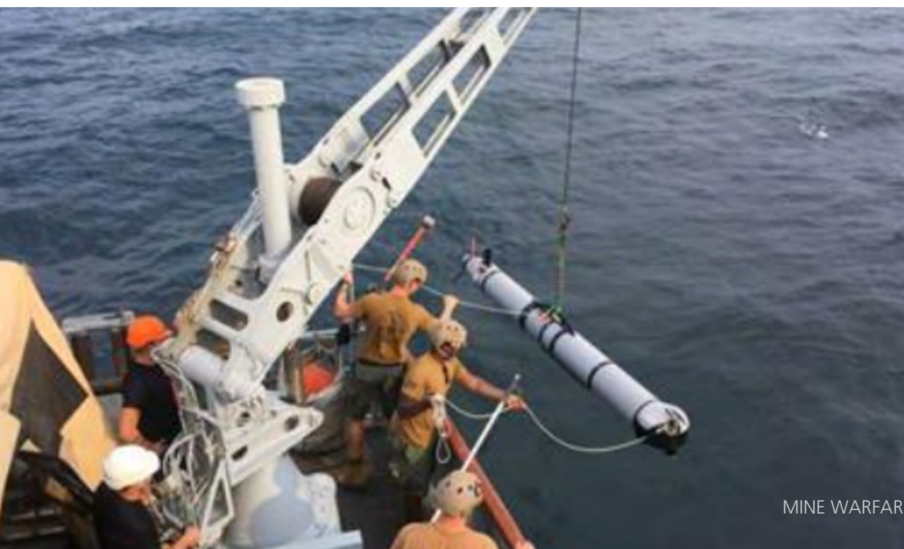
Figure 1 – UK and US personnel deploying a US Mk18 Mod II UUV from HMS BROCKLESBY
