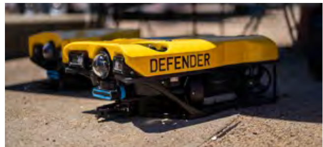
Fig 7. Defender ROV (image courtesy of Videoray)
