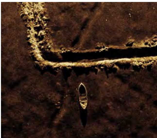
Fig 6. Kraken MinSAS image of anchor scour and sunken dinghy (image courtesy of Kraken Robotics)
