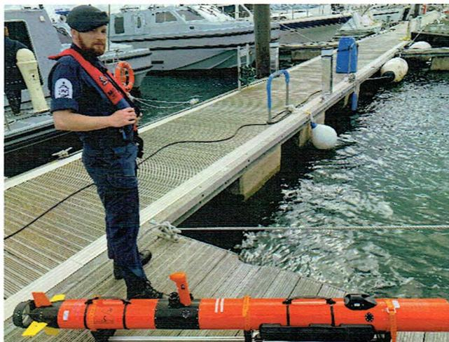
AUV Mission Operator, ABMW Ewart preparing an IVER3 for deployment
